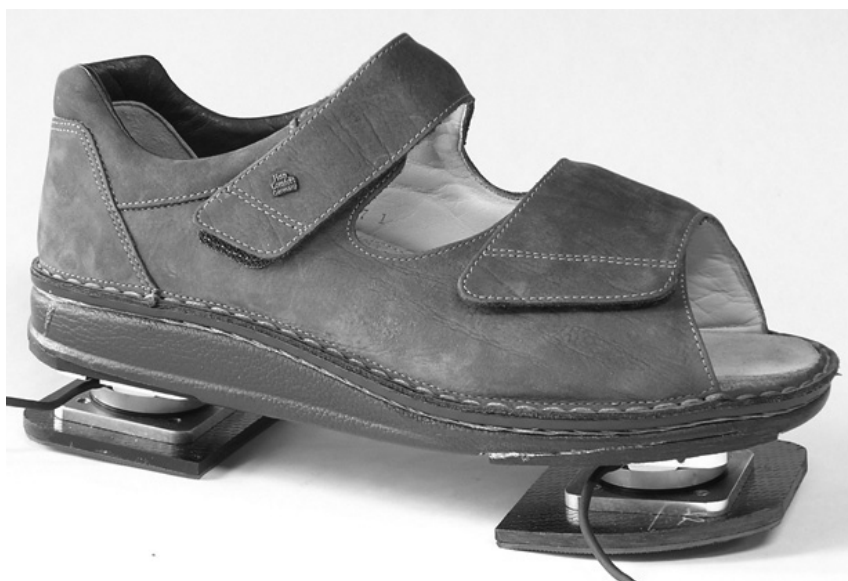
Figure 1.7: Picture of the instrumented shoe with two 6D force/moment sensors beneath the heel and the forefoot proposed by Veltink et al. [36].
