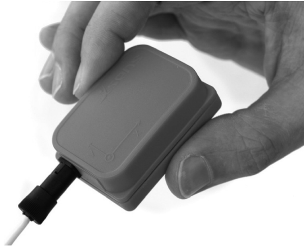
Figure 1.4: Inertial and magnetic sensor (MTx, Xsens Technologies B.V. [20]).
