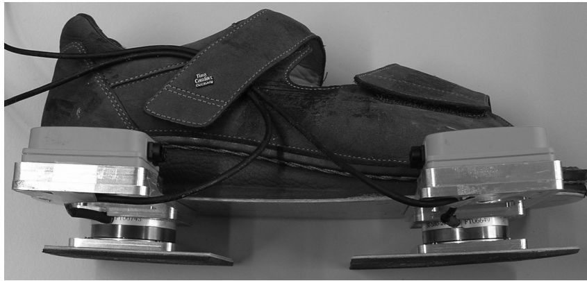
Figure 4.1: Picture of the instrumented shoe with force/moment sensors beneath the heel and forefoot and inertial sensors rigidly attached to the force/moment sensors.
