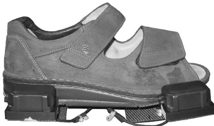
Figure 2.1: Instrumented shoe with force transducers, and inertial sensors.
