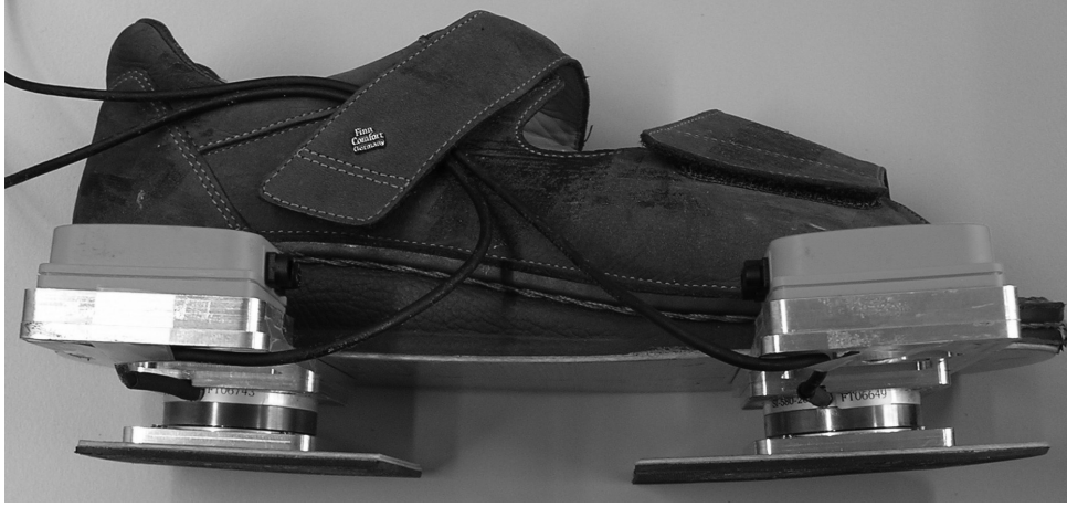
Figure 3.1: Picture of the instrumented shoe with force/moment sensors beneath the heel and forefoot and inertial sensors rigidly attached to the force/moment sensors. A thin flexible glass-fiber plate connects both sensors allowing regular flexion of the foot during push-off.
